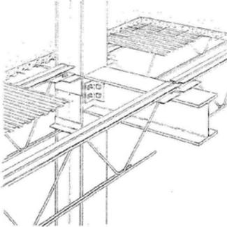
Table below lists costs for a floor system on steel columns and beams using open web steel joists, galvanized steel slab form, and 2-1/2" concrete slab reinforced with welded wire fabric.
