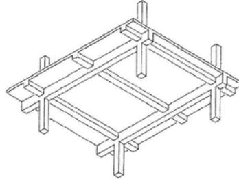
**General:** Solid concrete one-way slab cast monolithically with reinforced concrete support beams and girders.
