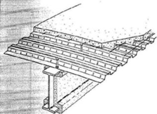
**Description:** Table below lists costs (\$/S.F.) for a floor system using composite steel beams with welded shear studs, composite steel deck, and light weight concrete slab reinforced with W.W.F. Price includes sprayed fiber fireproofing on steel beams.
